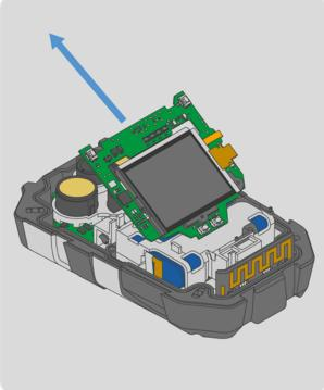
4. Lift the display PCBA and display assembly away from the main board at the angle shown.
