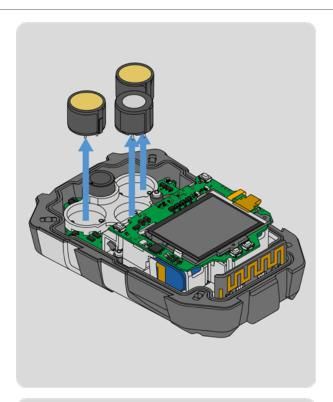
5. Remove the sensor(s) you plan on replacing by pulling it up and clear of the bracket.
