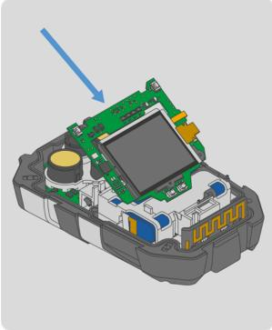
5. Take the new display PCBA and display assembly, and insert the bottom left edge under the snap fit on the battery holder. Push the display PCBA down to engage the board to board connector.
